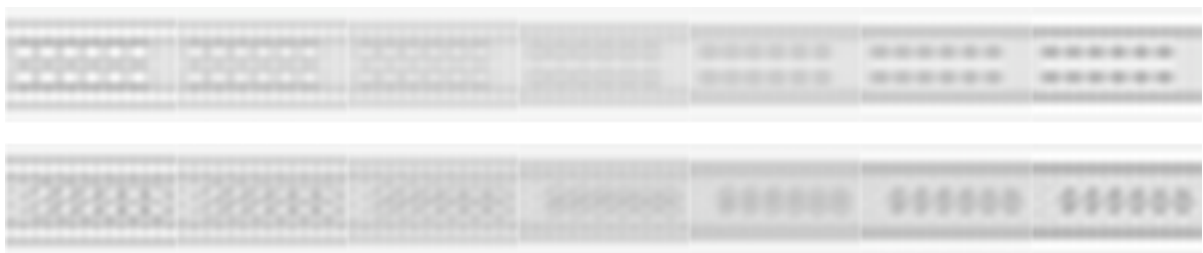
FIG 3. Calculated focal series using the JEMS program by P. Stadelmann. Top: the molecule in standing position. Bottom: the molecule in lying position. Simulations were made with constant thickness of 2 nm and defocus step of 1 nm.
