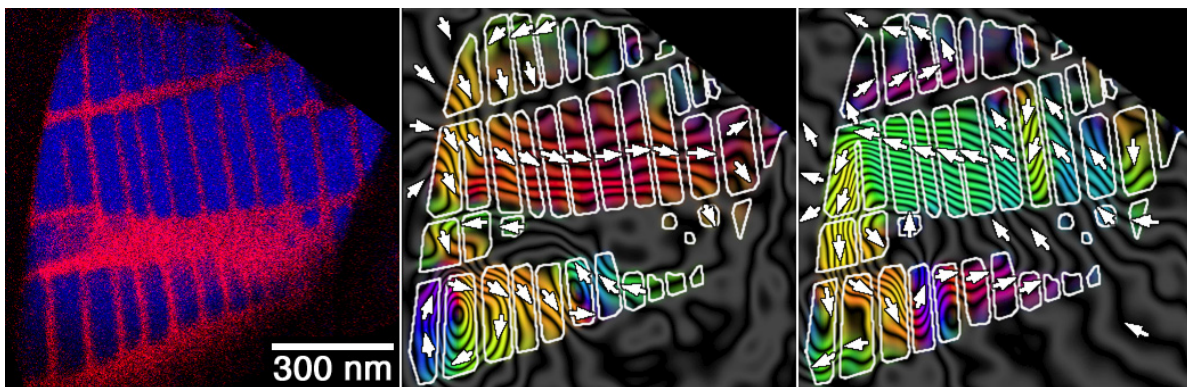
Figure 7. (a) Chemical map of naturally occurring titanomagnetite, obtained using a Gatan imaging filter. Blue regions show magnetite ( \text{Fe}_3\text{O}_4 ) blocks, which are separated from each other by paramagnetic ulvöspinel ( \text{Fe}_2\text{TiO}_4 ). (b) and (c) show magnetic phase contours measured using electron holography from the same region, acquired after magnetizing the sample in different directions using the magnetic field of the microscope objective lens. The colors show the directions of the magnetic induction.
