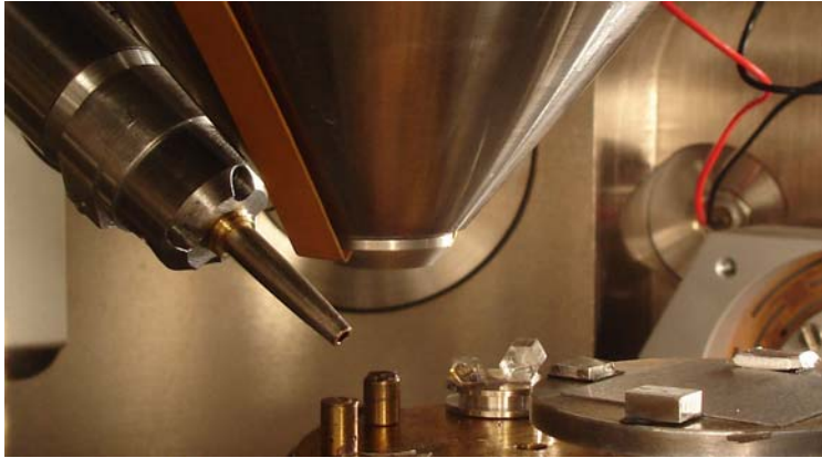
Figure 1. X-ray optics inside the SEM chamber
