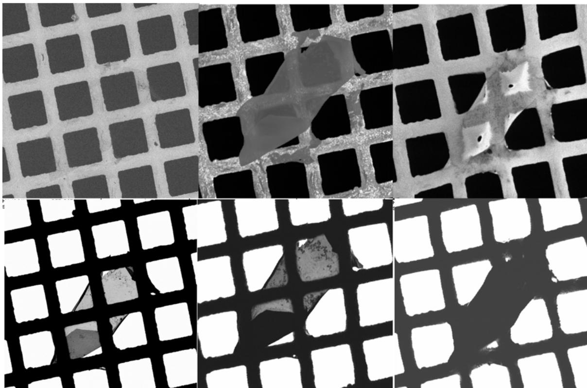
**Figure 1:** 10 nm carbon foil on a 25  $\mu\text{m}$  period Cu grid: reflected electron micrographs (upper row) and transmitted electron images (lower row), electron energies from the left: 6 000 eV, 400 eV, 20 eV.
