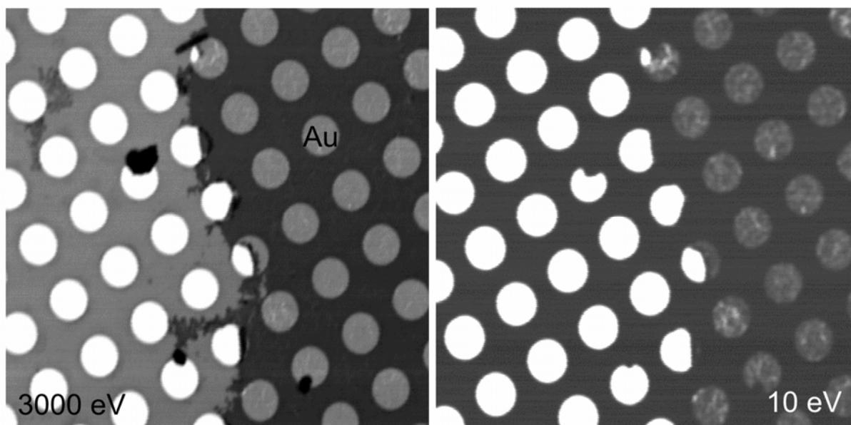
**Figure 2:** Transmitted electron micrographs of the Quantifoil (holey carbon film of 12 nm in thickness with round holes of 2  $\mu\text{m}$  in diameter) with the right part covered by a 3 nm gold film.
