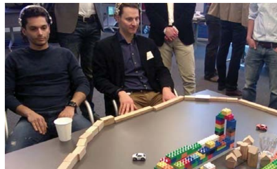
Figure 1. A picture taken during the BCI racing game. The two opponents wearing the wireless headset are in the upper left corner, the white and orange remote controlled cars are driving on a racetrack on the table.
