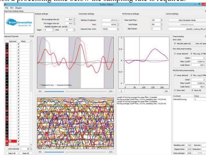
**Figure 1.** User interface of Turbo-Satori. The user is able to inspect channels in detail and combine them in one view. All preprocessing parameters can be adjusted in on-line and are accessible during data acquisition. A log window shows current information.
