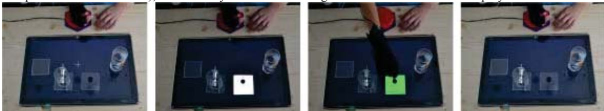
Figure 1: Paradigm: Participants were instructed to rest the hand comfortably on a pressure button. At second 0, a cross appeared on the screen to focus users' attention. At second 2, one of the objects was highlighted in white for a random time period. As soon as the highlighting turned green, participants performed the reach and grasp tasks and held the object as long as the green highlighting remained. Thereafter participants returned their hand to the pressure button.
