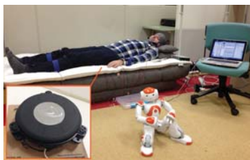
Figure 1. The fbBCI user lying on a mattress with tactile transducers embedded. NAO robot depicted seating is controlled using the fbBCI. One of the tactile transducers used in experiments is depicted in the lower left panel.
