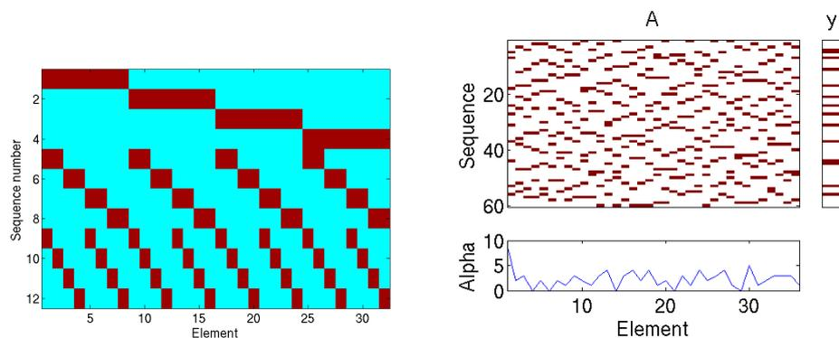
Figure 1: Left: template for a 36-element grid and 1-in-4 flash-rate. Each line represents the flashing elements  $\mathbf{a}(t)$ . Right: example of accumulation based on the randomized grid on the left, over 60 flashes, with element 1 as target.
