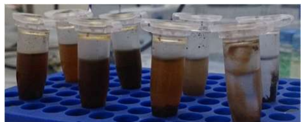
Fig. 1. Examples of dissolved lignin in various solvents after centrifugation.
