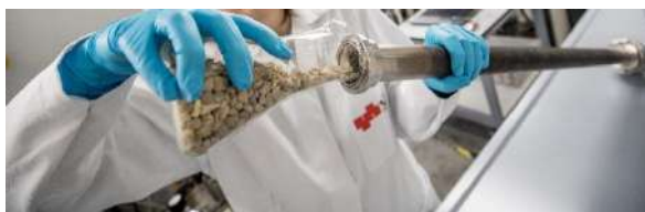
Fig. 1: Tubular reactor being filled with iron ore sample from the Styrian Erzberg
