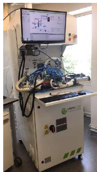
Fig. 2: Greenlight G60 fuel cell test station and main system specifications for single PEM fuel cell testing on laboratory scale.
