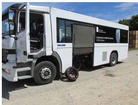
Figure A.2.: test truck for lateral tire force parametrization [87].
