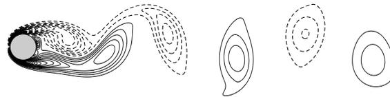
Figure 6.12.: Vorticity contours for the flow around a cylinder at  $Re$  100
