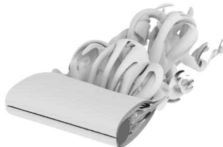
Figure 6.17.: Magnitude of vorticity around a 3D cylinder for Re 400 obtained with a TRT-LES simulation
