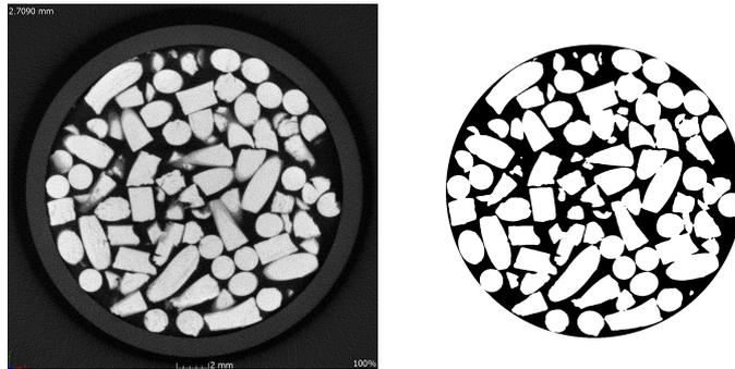
Figure 7.1.: Micro-CT scan and enhanced computational domain: Raw scan (left) and processed image (right)
