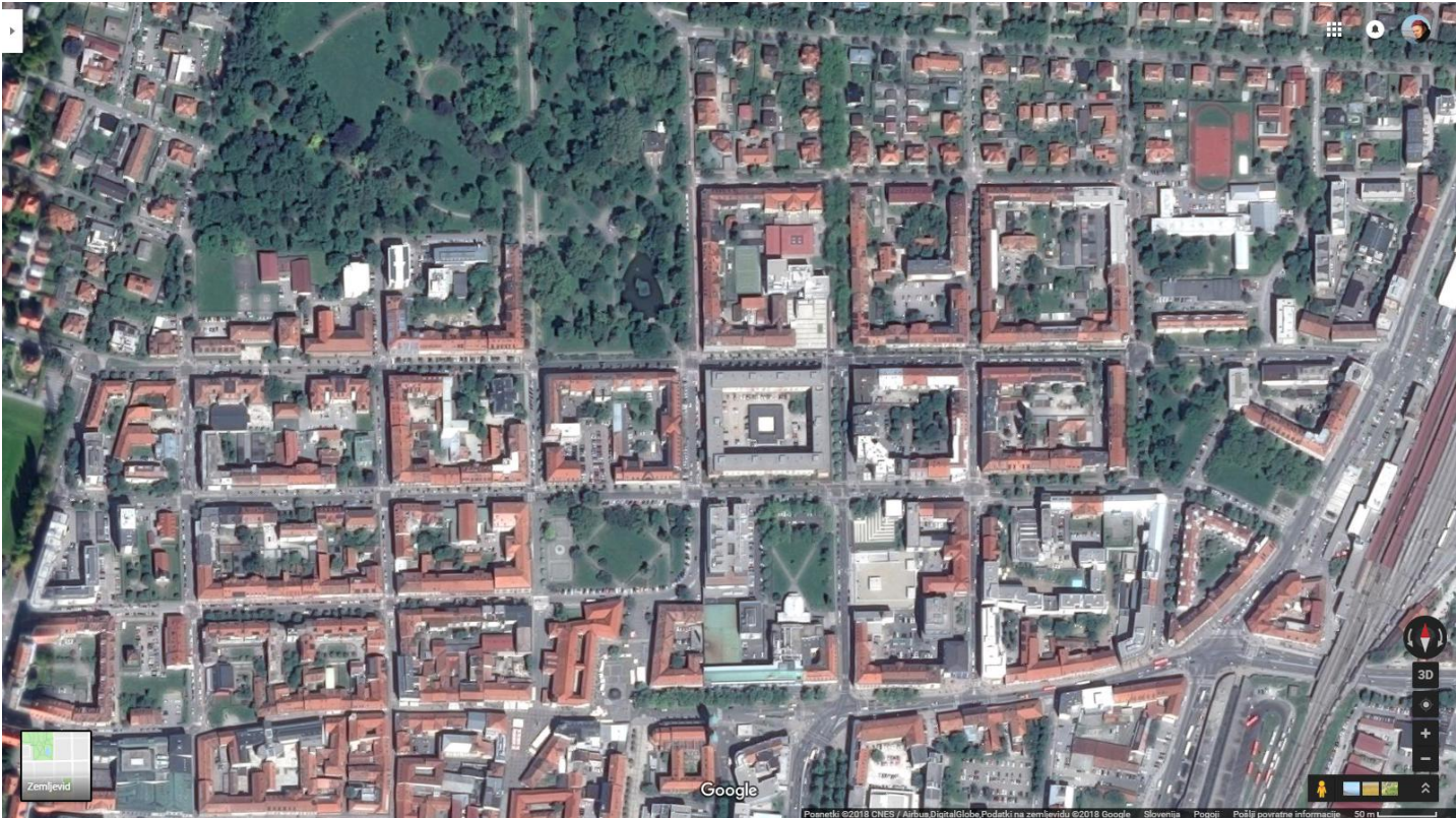
Fig. 6.9 Maribor, Slovenia. The Gründerzeit city extension is attached to the northeastern corner of the medieval structure and consists of closed urban blocks, regulated by the main streets, developed from the core structural principles. Google Maps, ©2018 CNES / Airbus, DigitalGlobe
