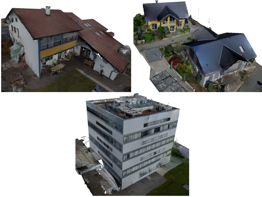
Figure 5.1: Results of the proposed approach textured with [93]. One can observe that planar parts in the scene (façades, windows, roof) are represented by planar surfaces and building edges where two façades intersect each other are represented by straight lines. Note that holes in the model are due to missing visibility information during texturing.
