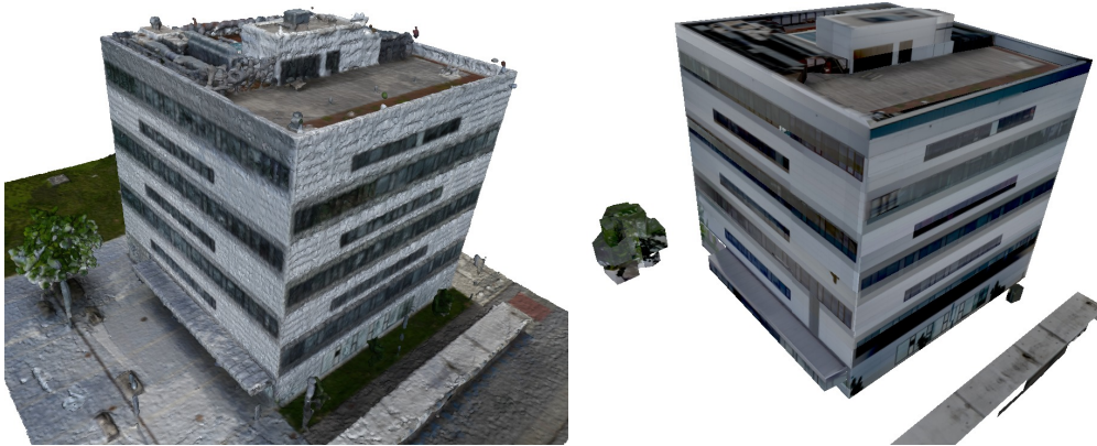
Figure 6.9: Meshed dense 3D reconstruction and resulting regularized model of the block building. Left: A 3D building reconstruction, for which a dense point cloud was reconstructed with Sure [79], which was finally meshed using Poisson surface reconstruction [43] (visualized with vertex coloring). Such a mesh can be used as input for our approach. Right: Resulting regularized model from our pipeline with line+mesh smoothing, textured with [93]. We deliver clean and smooth surfaces where the meshed dense point cloud contains a lot of noise. The parameters were set to: \lambda_{mesh} = 0.4 , \lambda_{lines} = 0.1 and d = 50 .
