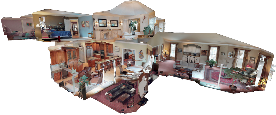
Figure 1.3: Reconstruction of an indoor scene with Matterport [59]. Matterport creates 3D models from indoor and outdoor scenes using an active 3D scanning device, like a structured light or a laser scanner. After being processed, the user can explore the scene using a VR device or in the browser. Image from Pennsylvania Craftsman Home, taken from [59].
