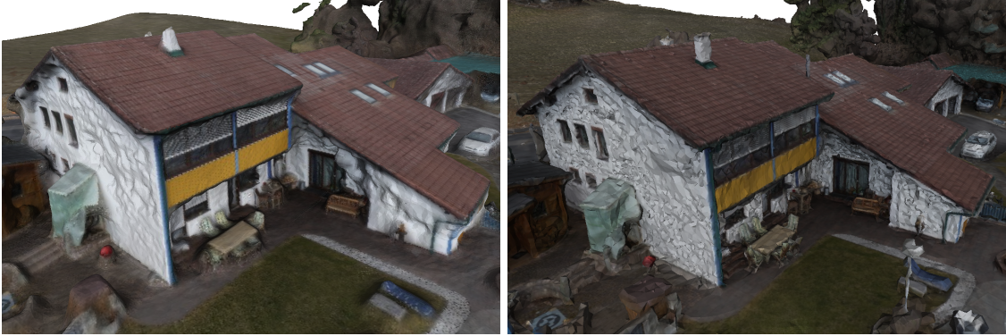
Figure 1.1: Example reconstruction results from commercial reconstruction software: Agisoft [1] (left) and Pix4D [75] (right). Using images taken from an Unmanned Aerial Vehicle (UAV) as input, these two commercial 3D reconstruction pipelines can reconstruct the scene accurately and with high detail. However, especially at poorly textured façades, the reconstructed surface gets very noisy. Further, edges of the building are reconstructed very smooth and not as sharp edges, with would be favored for buildings with planar shapes.
