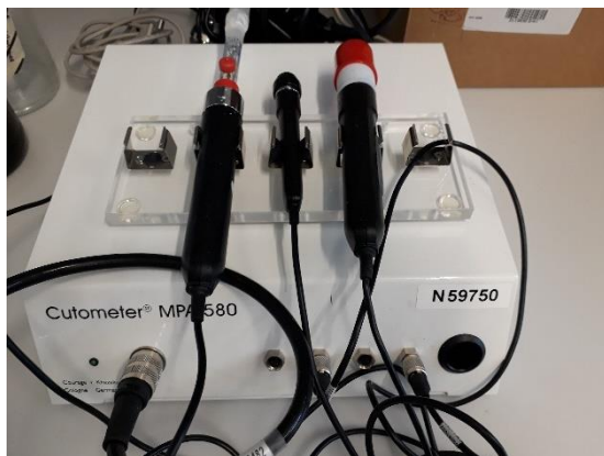
Figure 6: Cutometer MPA580 from Courage + Khazaka used for the skin measurements.
