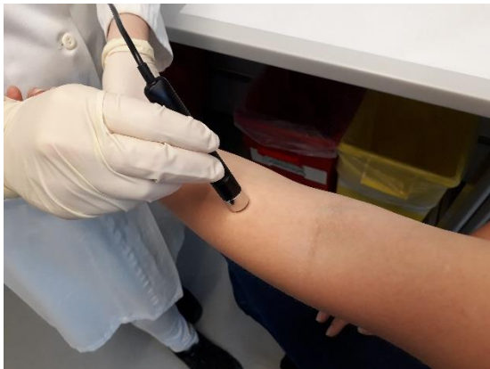
Figure 10: Cornemeter measurement procedure with the CM825 Courage + Khazaka for determination of skin moisture.
