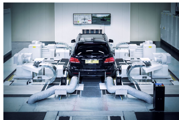
(b) R2R full vehicle test bed.
