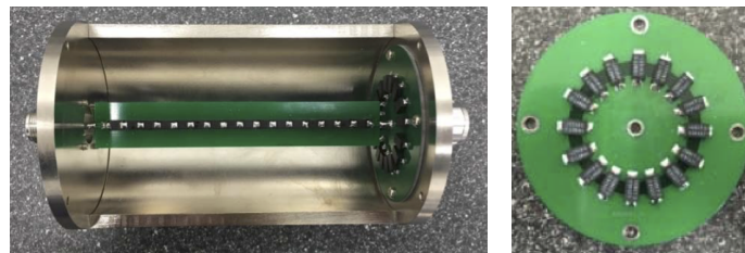
Figure 1.11: Serial (left) and parallel (right) connected identical resistors for voltage dividers at NIM China by Shi et al. [Shi+18a], © 2018 IEEE.
