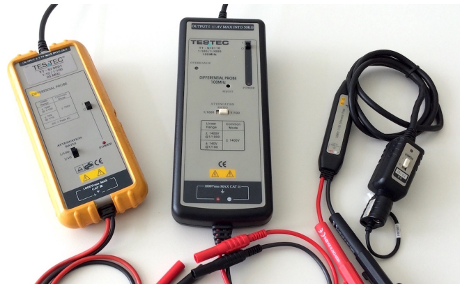
Figure 1.12: Examples for commercially available high voltage differential probes. From left to right: Testec SI-9001 (low-cost probe, 25 MHz bandwidth, \pm 700 V), Testec SI-9110 (high-bandwidth probe, 100MHz bandwidth, \pm 1400 V differential input voltage) and Testec SI-51 (high-accuracy and small-size probe, 50MHz bandwidth, \pm 700 V differential input voltage, \pm 1 % accuracy).
