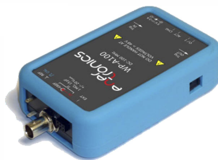
Figure 1.16: Wireless Bluetooth oscilloscope by Lobsiger et al. [Lob+14], © 2014 IEEE.
