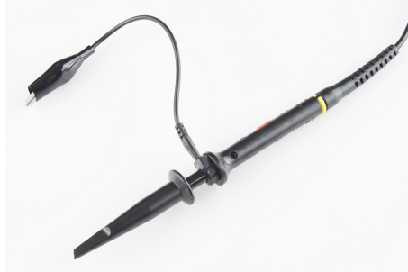
Figure 1.8: Standard passive oscilloscope probe for wide-band, single-ended voltage measurements (Photo: SparkFun, licensed under CC BY-SA 4.0).
