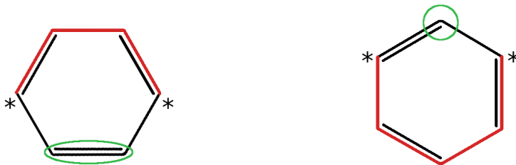
Fig. 1.2. Two diagrams resulting from the application of the graphical scheme discussed in the main text to a benzene molecule. The stars indicate the sites contacted to the electrodes.
