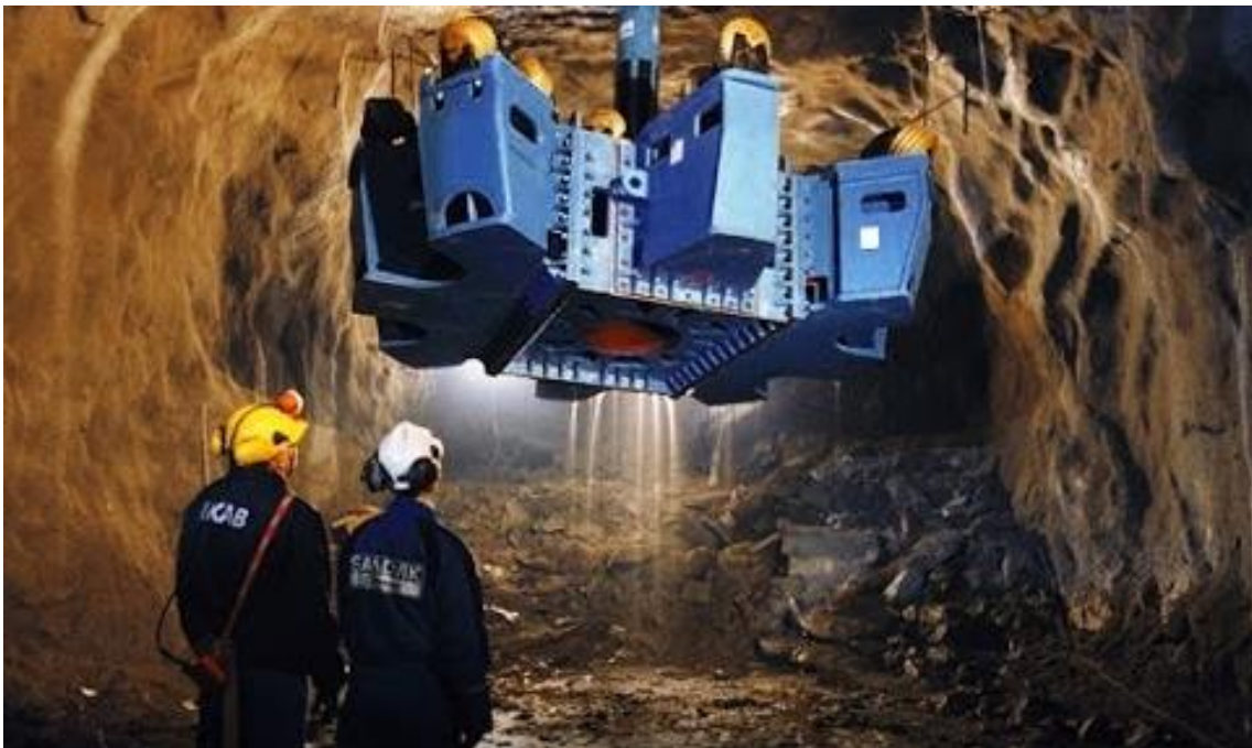
Figure 53: Reamer of a Raise Boring Machine [38]
