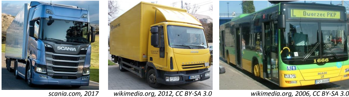
Figure 85. Examples for simulated HDV classes. F.l.t.r.: Tractor-trailer, delivery truck, rigid city bus
