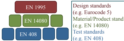
Fig. 3 Sketch of the 3-step pyramid applied in internat. standardization for the construction sector
