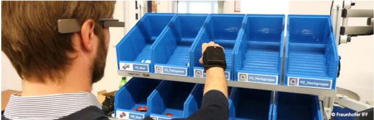
Figure 7: Combined use of HMD and RFID Wristband in a first experimental setup (source: Fraunhofer IFF)
