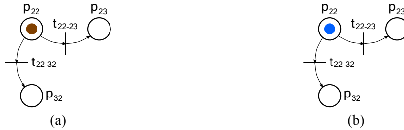
Figure 8: Detail of the CPN representing the section of the \pi -conveyor: movement from cell #22 to cells #23 (eastbound) and #32 (southbound).
