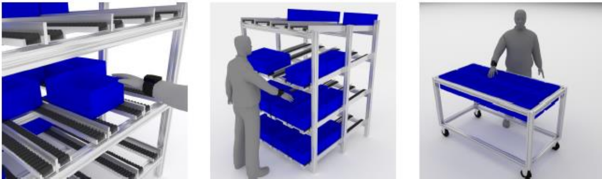
Figure 6: Typical use cases. (a) control of storage, (b) control of picking, (c) control of putting (source: Fraunhofer IFF)
