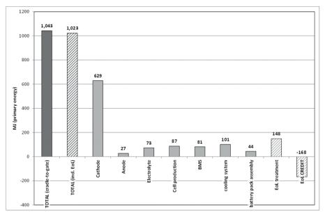
**Figure 2** – Cumulative energy demand (CED) per kWh of battery energy capacity, with and without end-of-life (EoL), and highlighting the individual contributions of the main components.
