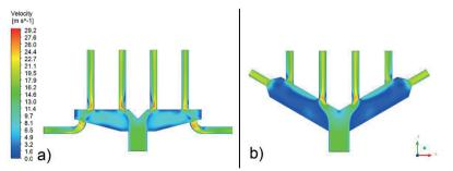
Figure 6. Comparison of the velocity in case of the standard air manifold (a) and the prototype (b): 3D analysis, symmetry plane, inlet velocity of 12.5 m/s.
