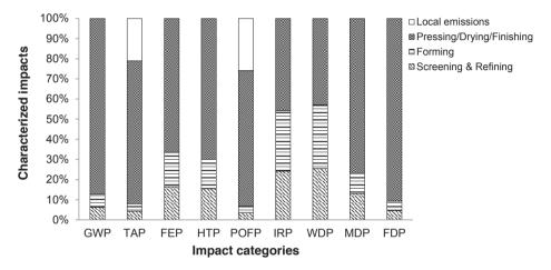
Figure 3.3. Breakdown of Recipe Midpoint (H) characterized impacts for different steps of the paper production phase, referred to a functional unit of 1 ton of produced paper.
