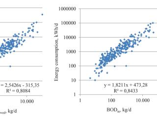
Figure 3.3. Electric energy consumption referred to BOD removed, KPI<sub>BODremoved</sub>.
