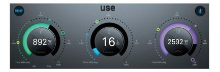
Figure 3.1: As visualized on the in-home display; real-time feedback on consumption of electricity (left), hot tap water (center), and heating (right), accompanied by historical (green ring) and normative (yellow ring) comparisons. By clicking on the icons monthly, weekly, and hourly feedback will be visible.
