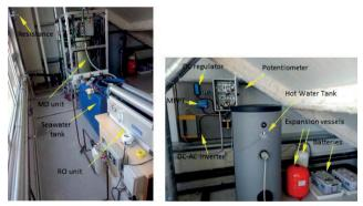
Figure 2.2: Detail of the RO and MD units (left) and electric cabinet, hot water tank and batteries.
