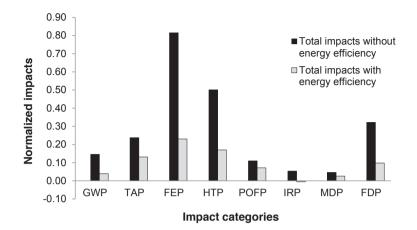
Figure 3.4. Recipe Midpoint (H) normalized impacts without and with energy efficiency implementation, referred to a functional unit of 1 ton of produced paper.
