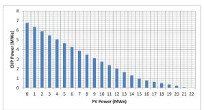
Figure 3 CHP power needs to balance the export and import electrical energy depending on the PV power installed
