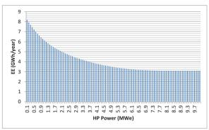
Figure 5 Electrical energy exported to the national grid as a function of HP power installed
