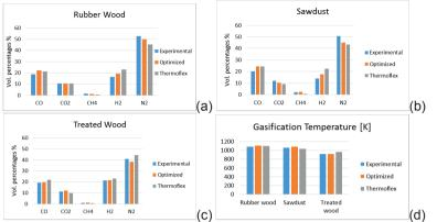
Figure 2.2: Comparison between experimental measurements, numerical results of both the optimized equilibrium model and the Thermoflex<sup>TM</sup> model in terms of volumetric syngas compositions for a) rubber wood, b) sawdust, c) treated wood and d) gasification temperature.
