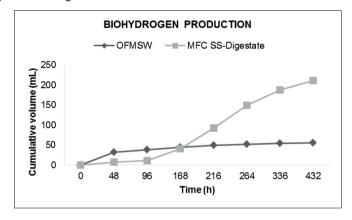
Fig.3: Cumulative  $BioH_2$  production over time. OFMSW: solid residues from the OFMSW. MFC SS: Microbial Fuel Cell Solid Substrate
