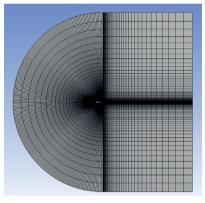
Fig. 1: Mesh generated for the airfoil section
