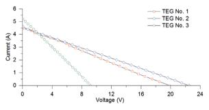
Figure 3: I-V characteristics of the thermoelectric generators.
