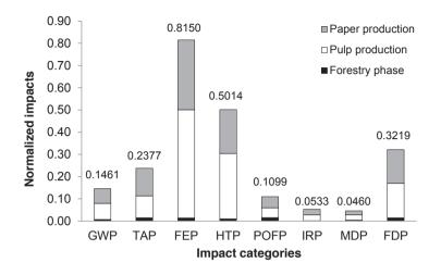
Figure 3.1. Recipe Midpoint (H) normalized impacts calculated for the pulp and paper mill, referred to a functional unit of 1 ton of produced paper.
