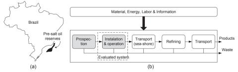
Figure 1. (a) Location of the pre-salt oil reserves in Brazil; (b) Process existing in the pre-salt oil extraction (dashed lines indicate the evaluated system in this work).
