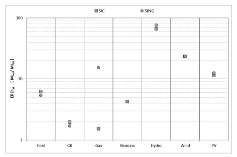
**Figure 1** - EROI<sub>el</sub> results per technology (N.B. values expressed as MJ of <u>electricity</u> output per MJ of <u>primary energy</u> investment).
