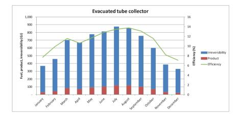
Figure 3.4: Aggregated monthly fuel, product, irreversibility and efficiency of evacuated tube collector.
