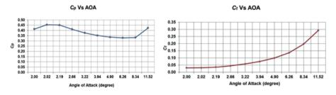
Fig. 3: Power coefficient  $(C_p)$  (left) and Thrust coefficient  $(C_t)$  versus angle of attack (AOA)
