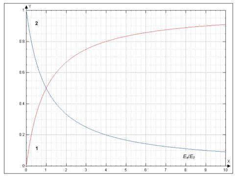
Fig. 1. Added energy index, equation (1) - 1, and sustainability index, equation (2) - 2, as functions of added energy.
