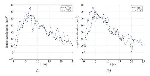
Fig. 3: Average time-histories of impact vertical acceleration acquired through PIV and ±200g piezoelectric accelerometer for: (a)  $\alpha = 0^{\circ}$  and  $\vartheta = 0^{\circ}$ , (b)  $\alpha = 10^{\circ}$  and  $\vartheta = 10^{\circ}$ .
