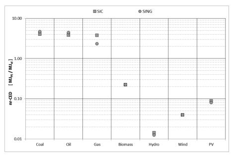
**Figure 2 -** nr-CED results per technology (N.B. values expressed as MJ of total <u>non-renewable primary energy</u> input per MJ of <u>electricity</u> output).
