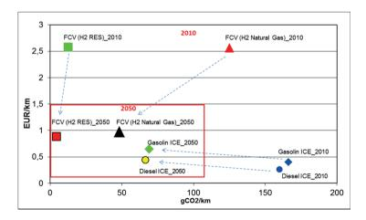
Fig. 3. Comparison of specific CO2 emissions and driving costs of FCVs and ICE vehicles in 2010 and 2050 (based on Ajanovic et.al., 2011)
