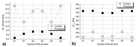
Figure 5. Distribution of selected outlet parameters in case of the basic air manifold and the prototype, inlet air velocity of 12.5 m/s
