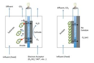
Fig.1: Schematic illustration of two-chamber and single chamber MFCs (Nastro R.A. et al., 2016).
