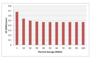
Figure 6 Electrical energy exported to the national grid as a function of the thermal storage capacity
