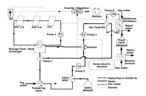
Figure 2.1: General structure of the polygeneration scheme.
