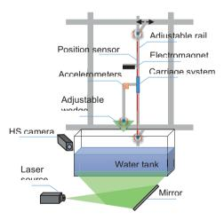
Fig. 1: Simplified sketch of experimental test bench
