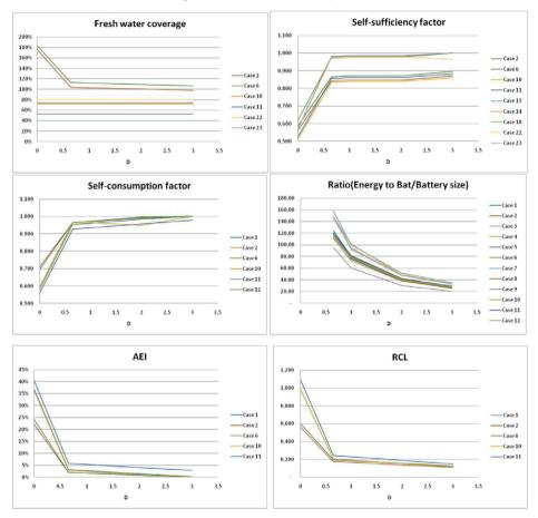
Figure 3.1. Fresh water coverage, self-sufficiency factor, self-consumption factor, equivalent number of cycles, AEI and RCL in different cases
