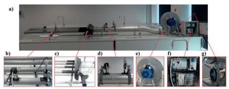
Figure 2. The test stand (a) and selected components: b) the outlet measurement set, c) the examined air manifold, d) the inlet measurement set, e) the centrifugal fan, f) the applied automation, g) the throttle.
