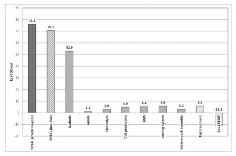
**Figure 3** – Cumulative greenhouse gas (GHG) emissions per kWh of battery energy capacity, with and without end-of-life (EoL), and highlighting the individual contributions of the main components.
