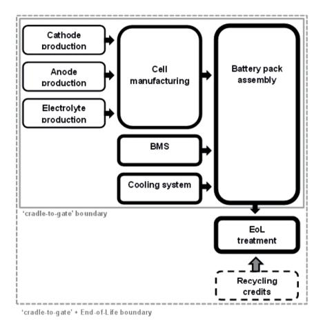
**Figure 1** – Flow diagram of the main steps in the manufacturing of a complete Li-ion battery pack, with indication of optional end-of-life (EoL) treatment and associated recycling credits.
