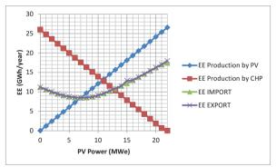
Figure 4 Electrical energy production by PV plants and by CHP plants, Electrical Energy imported by the national grid and Electrical Energy exported to the national grid.
