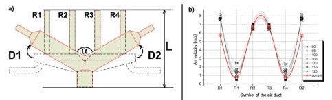
Figure 4. Proposed design of the prototype of the air manifold (a) and changes of the velocity on outlets from the manifold depending on value of the " $\alpha$ " angle (b).
