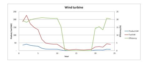
Figure 3.2: Time evolution of fuel, product and efficiency of wind turbine in an example winter day.
