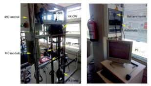
Figure 2.3: Detail of the internal hot water circuits (left) and control.
