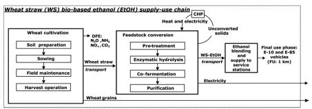
Fig. 1 System boundary of the wheat straw bio-ethanol (WS-EtOH) production-use chain in Campania Region. DFE: direct filed emissions;CHP: Combined Heating and Power-plant.
