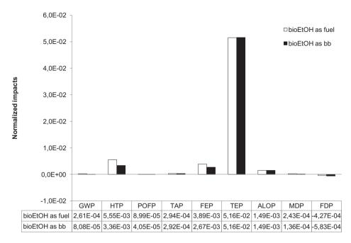
Figure 4.1. Recipe Midpoint (H) normalized impacts calculated for the use of bioEtOH as a fuel or as a building block (bb), referred to the functional unit of 1 kg of produced bioEtOH.
