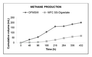
Fig.4: Cumulative methane production over time. OFMSW: solid residues from the OFMSW. MFC SS: Microbial Fuel Cell Solid Substrate.
