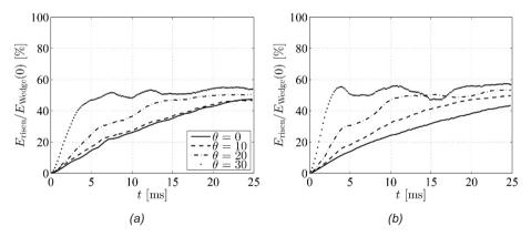
Fig. 4: Average of energy imparted to the risen water  $E_{risen}$  calculated as a percentage of initial wedge energy  $E_{wedge}(0)$  for: (a)  $\alpha = 0^{\circ}$ , (b)  $\alpha = 10^{\circ}$ . (Figures adapted from [10])
