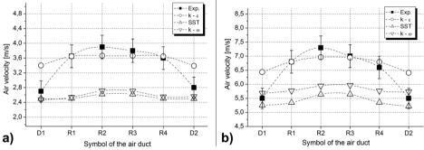
Figure 3. The comparison of results of the experiment and the CFD modelling for selected degrees of the throttle closing with different approaches to the simulation of the turbulence. R1 - R4 - primary air ducts, D1, D2 – secondary air ducts (see Fig. 8). Throttle closing in the given examples: a) 70%, b) 65%, c) 60%, d) 55%.
