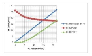
Figure 2 Electrical energy production by PV plants, Electrical Energy imported by the national grid and Electrical Energy exported to the national grid.
