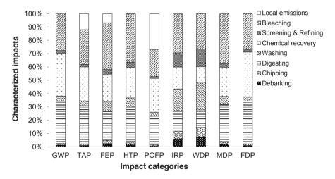
Figure 3.2. Breakdown of Recipe Midpoint (H) characterized impacts for different steps of the pulp production phase, referred to a functional unit of 1 ton of produced paper.
