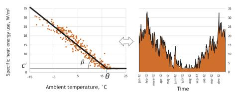
Fig. 1. Example of (left) the energy signature of a building and (right) specific heat energy use by time. Measured and modelled values are coloured orange and black, respectively.
