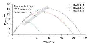
Figure 4: P-V characteristic of the considered thermoelectric generators
