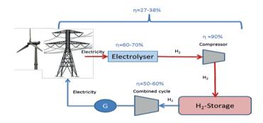
Fig. 5. Energy supply chains: Hydrogen as a storage for electricity from RES
