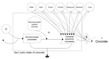
Figure 3.1: Simplified diagram of energy flows in the production of concrete.
