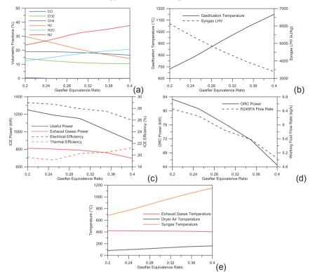
power of the ICE that reduces due to the lower primary energy content of the syngas, as well as on the thermal energy of the exhaust gases.
