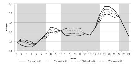
Figure 5.1: Potential load shift scenarios for a typical household in SRS, illustrating changes in intraday electricity consumption time patterns as an effect of 5%,10%, and 15% peak load reduction respectively (the light grey area represents the off-peak periods and the white represents the peak periods).
