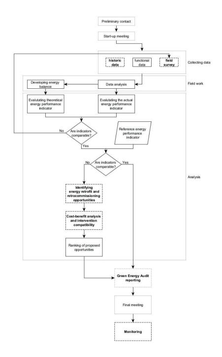
Fig. 1: the proposal process of energetic and environmental audit on historic building; grey square for elements described in UNI CEI EN 16247. The dashed lines represent the new elements introduced in
