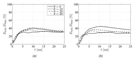
Fig. 5: Average of energy imparted to the fluid bulk  $E_{bulk}(t)$  calculated as a percentage of the total energy transferred to the fluid  $E_{fluid}(t)$  for: (a)  $\alpha = 0^{\circ}$ , (b)  $\alpha = 10^{\circ}$ . (Figures adapted from [10])
