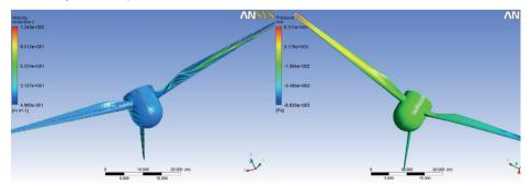
Fig. 6: The surface velocity streamlines (left) and 3-blade rotor colored by variable pressure forces
