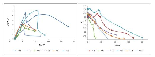
Fig. 5: Polarization an power curves after six weeks of operation at maximum power.
