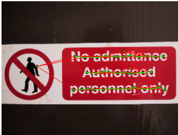
Figure 13. Region graph and its edge labeling corresponding to the best configuration (edges of the graph f(e) = 1 marked green, f(e) = 0 marked red)
