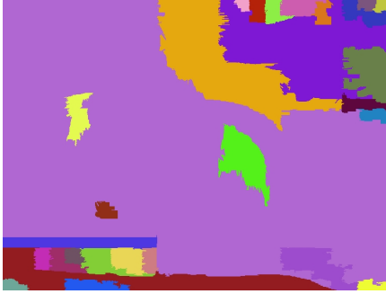
Figure 8. Post-processing error. If the post-processing is applied on a per cell-base, it is likely that the incremental approach creates very large superpixels covering nearly the complete image.
