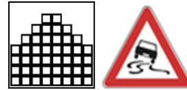
Figure 4. Arrangement of HOG cells in the detection window. The cell size is 6x6 pixels.
