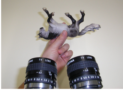
Figure 2. Stereo rig to capture the Graz-Stereo-Base-Eye database. We use two \mu Eye 1220C cameras and Cosmicar/Pentax lenses with a focal length of 12.5 mm. The baseline is approximately 6 cm (human eye distance), the vergence angle 5.5^\circ . The frame rate is 15 Hz. The size of the images is 480x752 px. For the calibration of the stereo rig we use the Camera Calibration Toolbox for Matlab [2]
