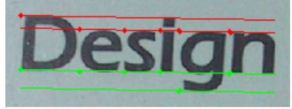
Figure 9. Sequence of characters cc with marked top (red) and bottom (green) points and text direction (top lines - red, bottom lines - green) obtained using the procedure la(cc)
