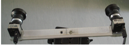
Figure 3. Stereo rig to capture the Graz-Stereo-Base-30 database. Focal length: 6.5 mm, Baseline: 30 cm, vergence angle: 6.5^\circ .
