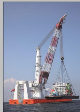
Heavy lift offshore crane MTC 78000
