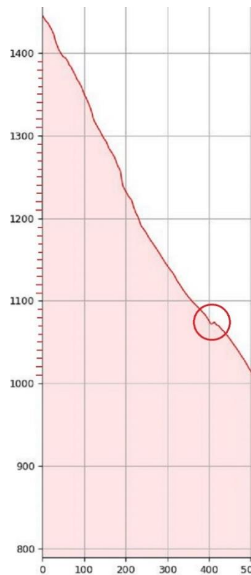
Figure 13: 2D cross-section through the active landslide derived from the GIS application QGIS (DTM), the elevation is over-scaled by 2:1. The red circle highlights the position of the protective dam.
