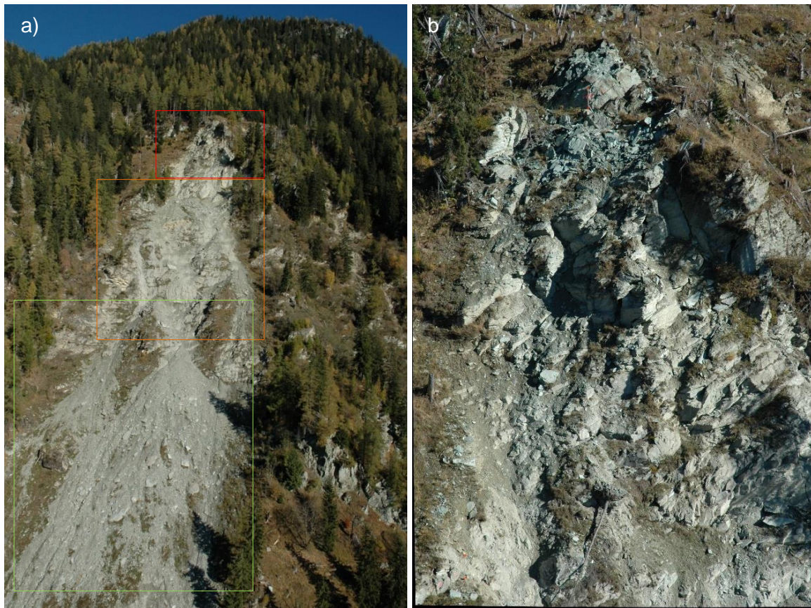
Figure 1: Photographs used for photogrammetry; a) impression of the whole active landslide (detachment area = red rectangle, transit zone = orange rectangle and accumulation zone = green rectangle), b) detailed image of the upper detachment area (Wieser et al. 2012).
