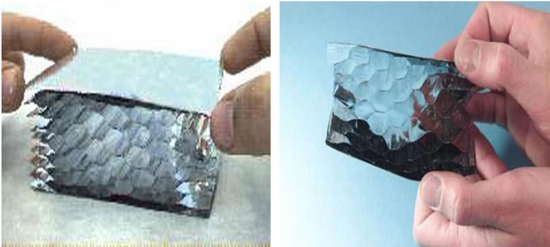
Figure 24. Puzzle structure and barrier foil of a GFP (Jelle, 2011)
