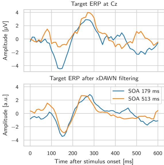
Figure 1: Averaged ERP waveforms elicited by auditory target stimuli delivered at time t=0 ms for two SOAs. Top: waveforms observed at channel Cz (no spatial filter was applied). Bottom: waveform observed after applying an xDAWN spatial filter.
