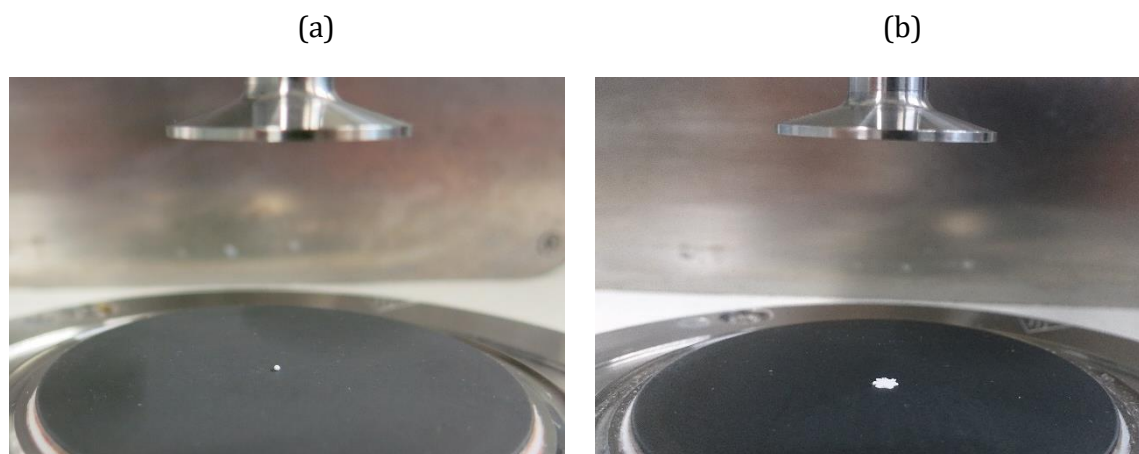
Figure 6. Microsphere on the rheometer plate (a) before and (b) after hardness test
