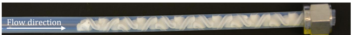
Figure 19. Foulant material on the elements of the 5.9 mm SM after the end of the precipitation experiment.
