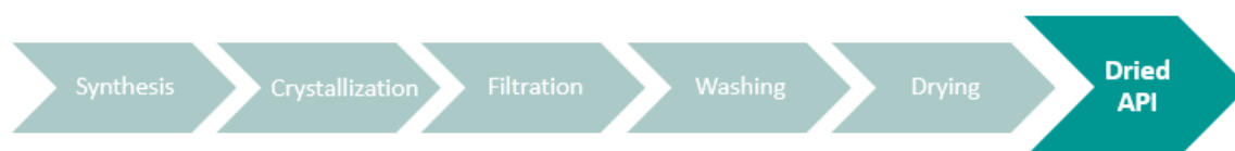
Figure 2. Process steps in primary manufacturing of pharmaceuticals.
