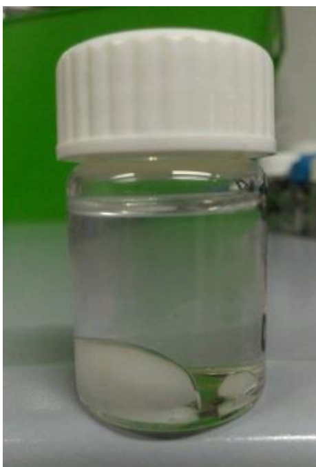
Fig. 6-4 Third phase in the solvent phase after the removal of the aqueous phase for formic acid with 25:25 TOA:1-octanol by weight, diluted in n -undecane; c_{\text{FA, initial}} = 0.8 mol/L; T = 25^\circ\text{C} ; ambient pressure
