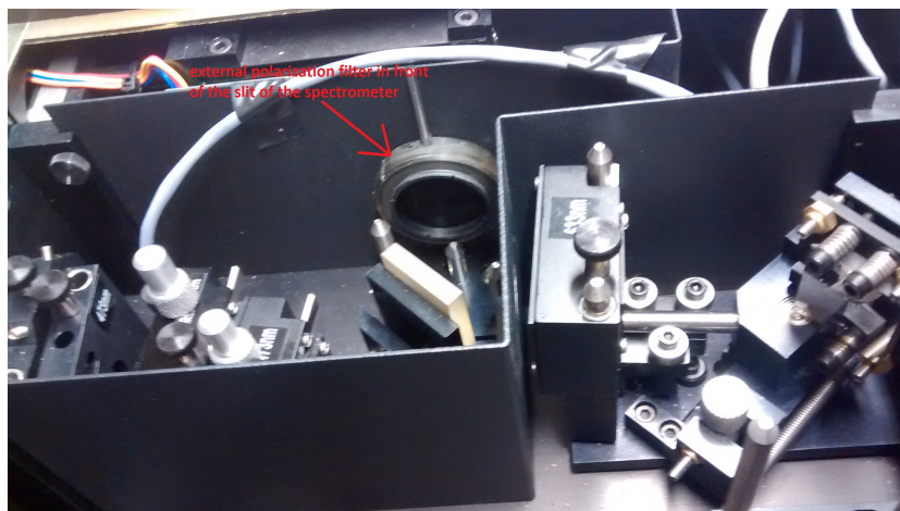
Figure 2.22: Improved setup for the measurement of Raman spectra with a polarized beam. A polarization filter is placed in front of the entrance slit of the spectrometer
