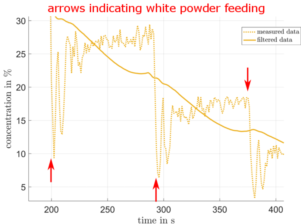
Figure 26: Close up of two feeding intervals with stepwise decrease in concentration.
