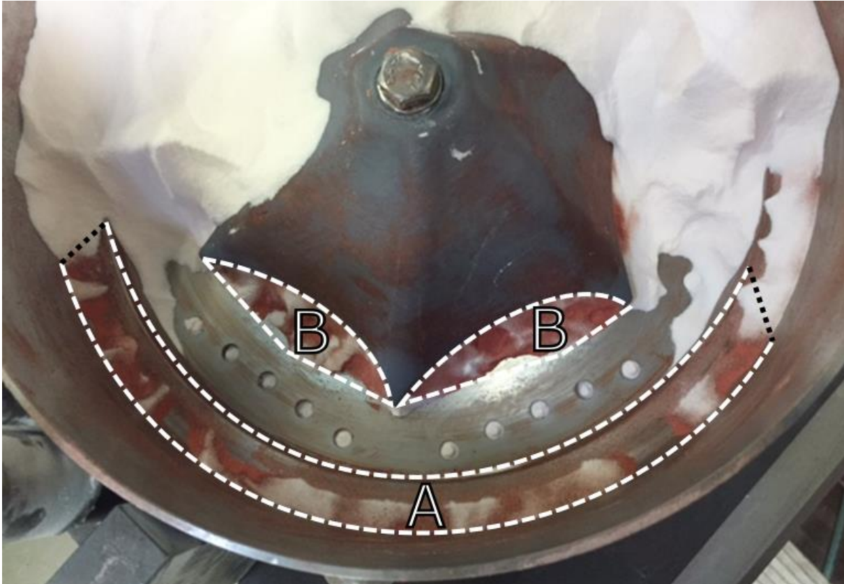
Figure 24: Stagnant zones revealed during cleaning (geometry 1, 110 tpm).
