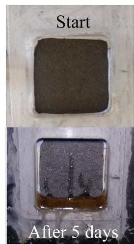
(b) Image of the backside of the electrode after start (top) and after 5 days (bottom).
