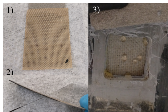
(b) Image of the backside (1) and side view (2) of the electrode after manufacture with the brown glass fiber cloth and image of electrode (E72) in the open set-up with the white glass fiber cloth (3).
