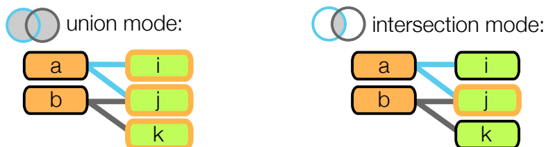
Figure 7.4: Illustration of the two highlight modes. In union mode, selecting items a and b highlights all items related to either of them, i.e., items i , j , and k . In intersection mode, only items related to both a and b are highlighted, which is item j in this case.
