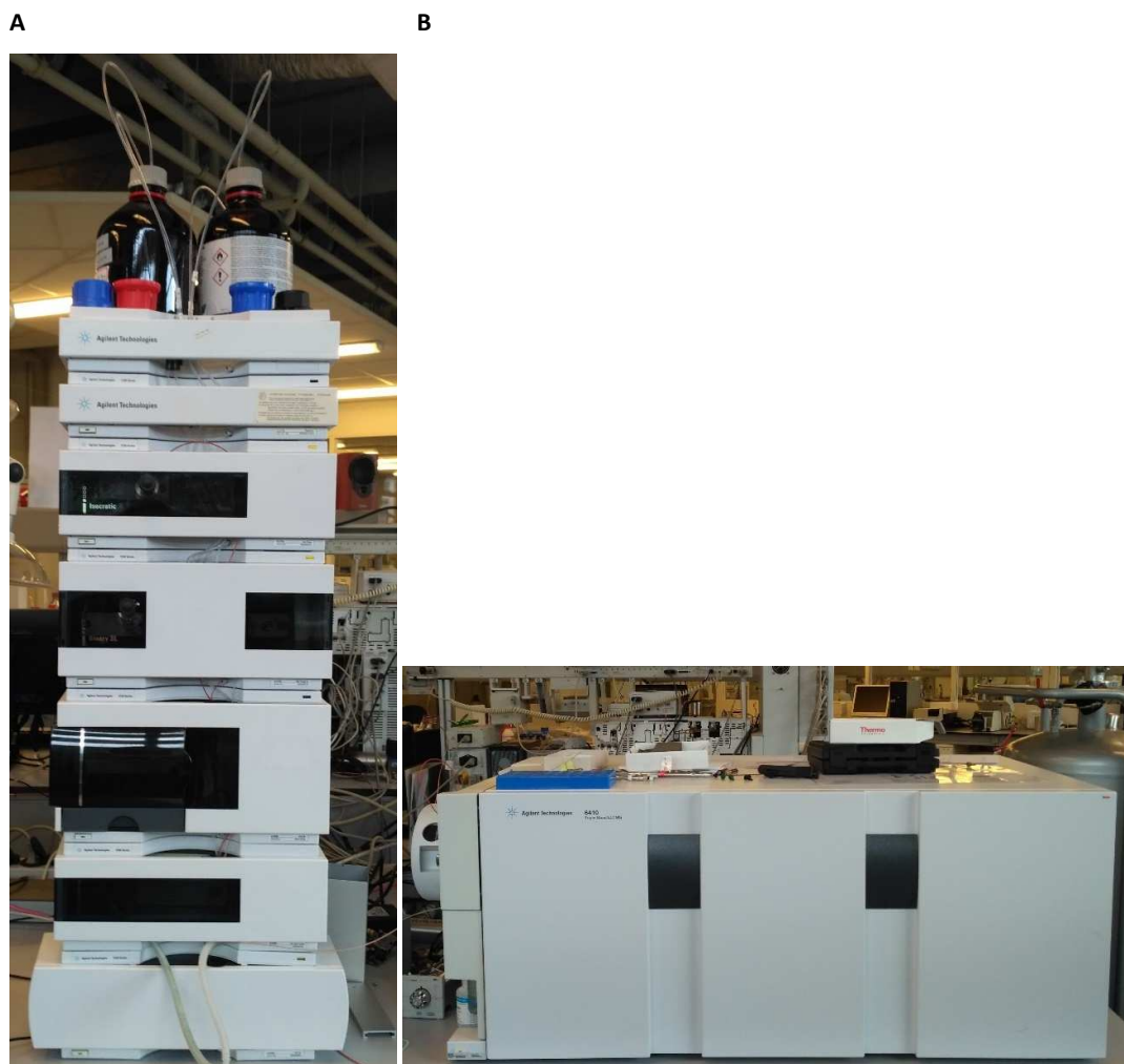
Figure 15: Agilent Technologies 6410 Triple Quadrupole LC-MS/MS; A: liquid chromatography B: triple quadrupole mass spectrometer
