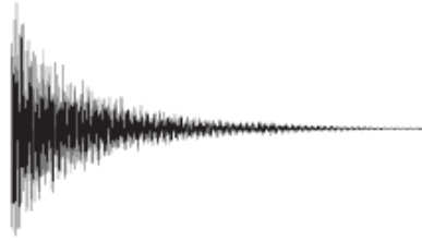
Figure 16. Example of a Free Induction Decay (FID). After the application of a rf-pulse the FID shows the highest amplitude and fades until the system is completely relaxed towards thermal equilibrium (Source: Clardige [64])
