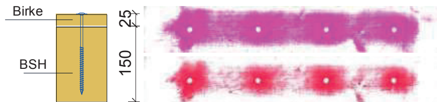
Abbildung 2-12: Birke | t = 25 \text{ mm} | d_{\text{head}} = 22 \text{ mm} [24]
