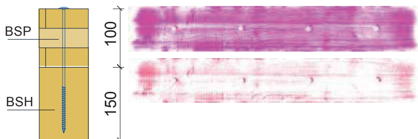
Abbildung 2-13: BSP | t = 100 \text{ mm} | d_{\text{head}} = 22 \text{ mm} [24]
