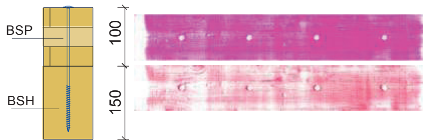
Abbildung 2-14: BSP | t = 100 \text{ mm} | d_{\text{head}} = 35 \text{ mm} [24]
