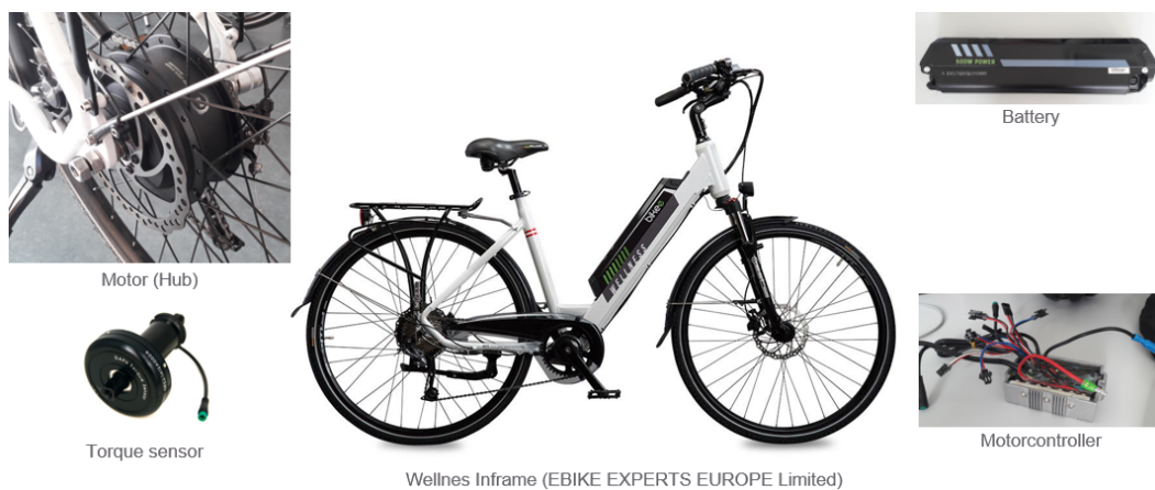
Figure 2.4: Main components of the used E-Bike
