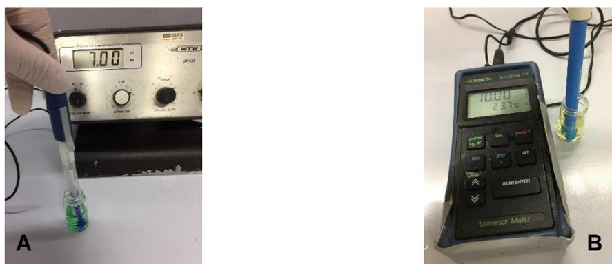
Figure 5-8: A; calibration of WTW pH522 at pH 7, B; calibration of WTW Multi. P4 at pH 10
