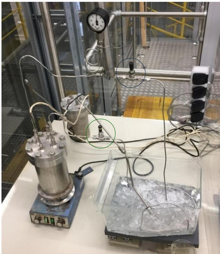
Figure 3-1: Picture of the experimental setup; cycles show the valves for the liquid (green) and gas (blue) sample lines
