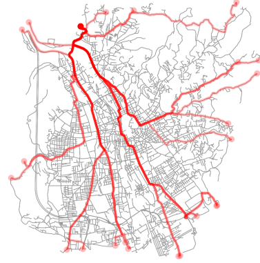
Figure 3.6: The shortest paths from node 318441610 in the road network of the City of Graz to the other entry nodes.
