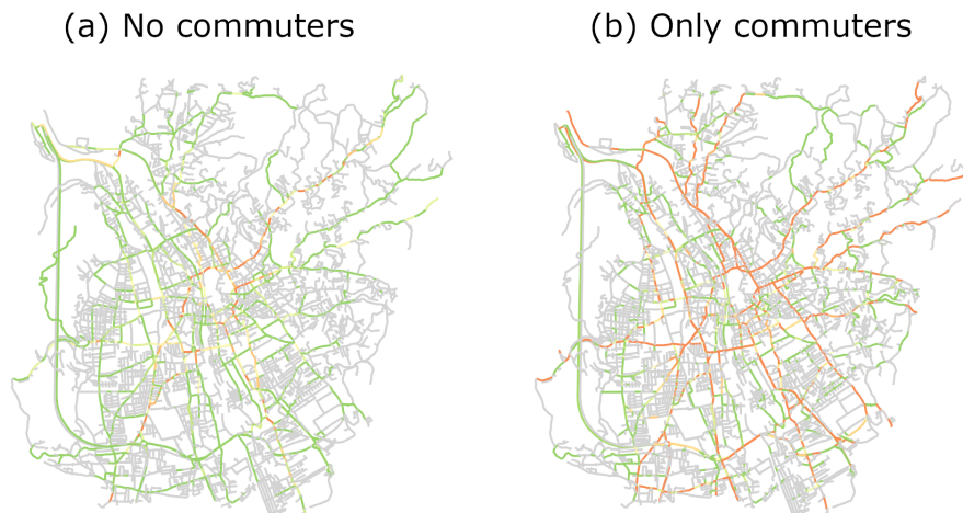
Figure 4.2: The congestion arising in a simulation of only the commuters (b) and without them (a) for the City of Graz.
