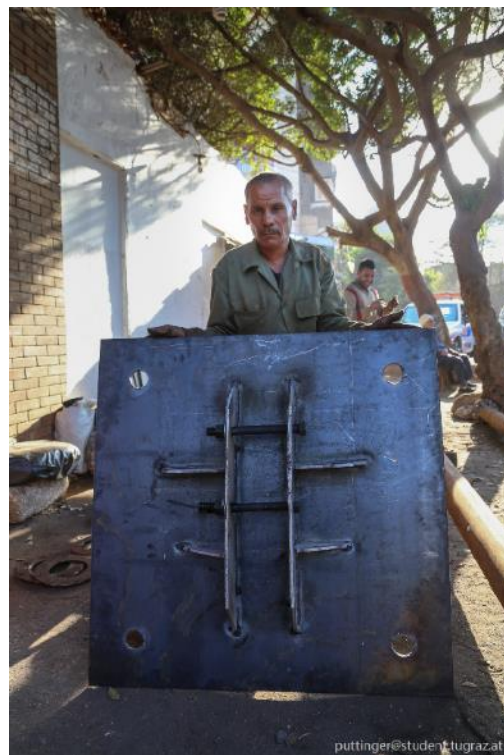
Figure 25: The heavy bottom plate which enables the lift (and lie down) of the mast
