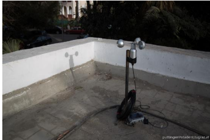
Figure 20: Test station of a logger prototype in Cairo.
