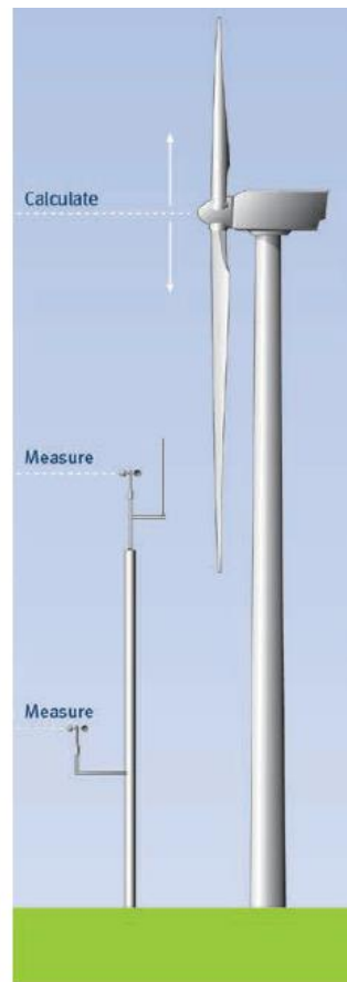
Figure 18: Measuring concept with an extrapolation of conditions in hub heights bigger than the mast. [18]
