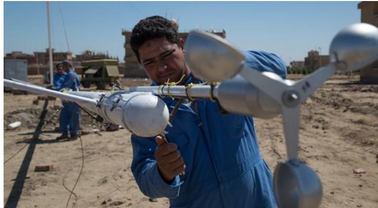
Figure 29: Assembling of the traverses with the sensors
