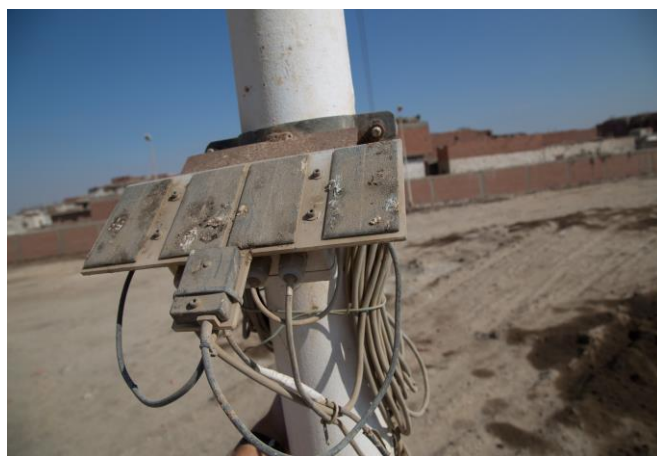
Figure 49: Data logger after a one-year measuring period. (at this time still in full operation)
