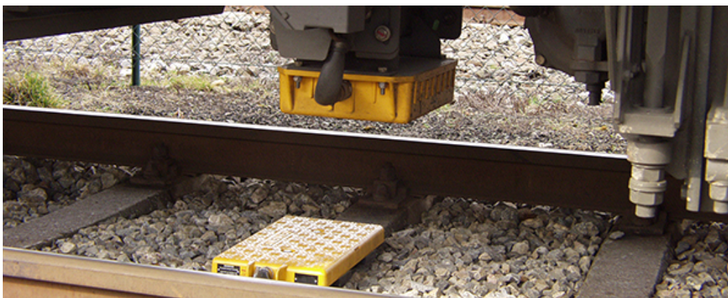
Figure 1.2: Balise system. The balise placed between the rails sends the actual position to the BTM passing over it [7].
