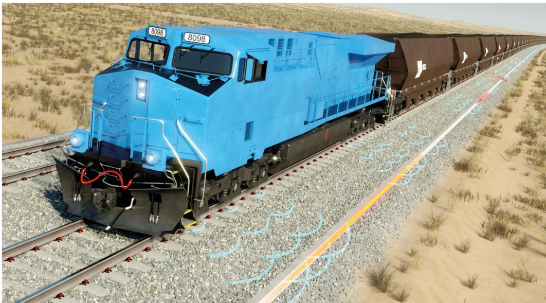
Figure 1.4: Vibrations generated by the train can be measured by a fibre optic cable buried near the track [11]. The sound waves travel from the rail's trough through the soil to the cable.
