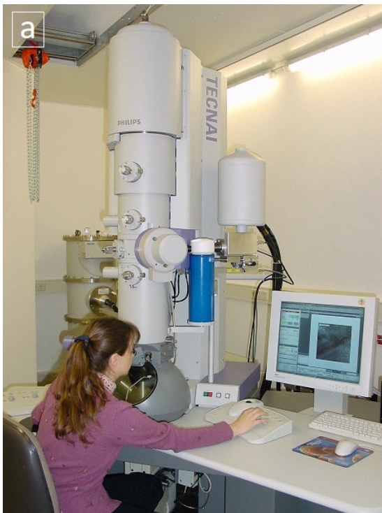
Figure 1.1: (a) FEI Tecnai G2 TF20 (by M. Wallner) (b) basic schematics of a TEM [36].
