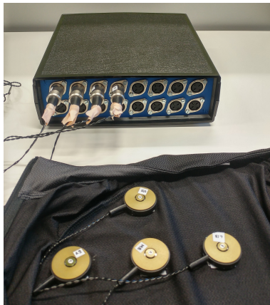
Figure 1: The stimulation device and tactor layout used in experiment 2. Inter-tactor spacing: 5-6 cm.
