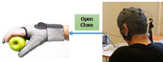
Figure 1: The envisioned BCI system for restoring grasping using a soft exoskeleton glove
