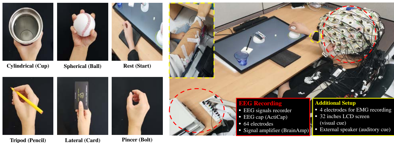
Figure 1: Description of the five grasping tasks and the experimental setup. (left) Five different reach-and-grasp tasks and the starting position. Five different grasping actions are matching to specific objects. (right) Experimental environment for EEG and EMG signals acquisition.
