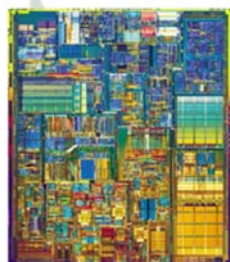
Pentium IV processor layout (Year: 2000, source: Intel)
