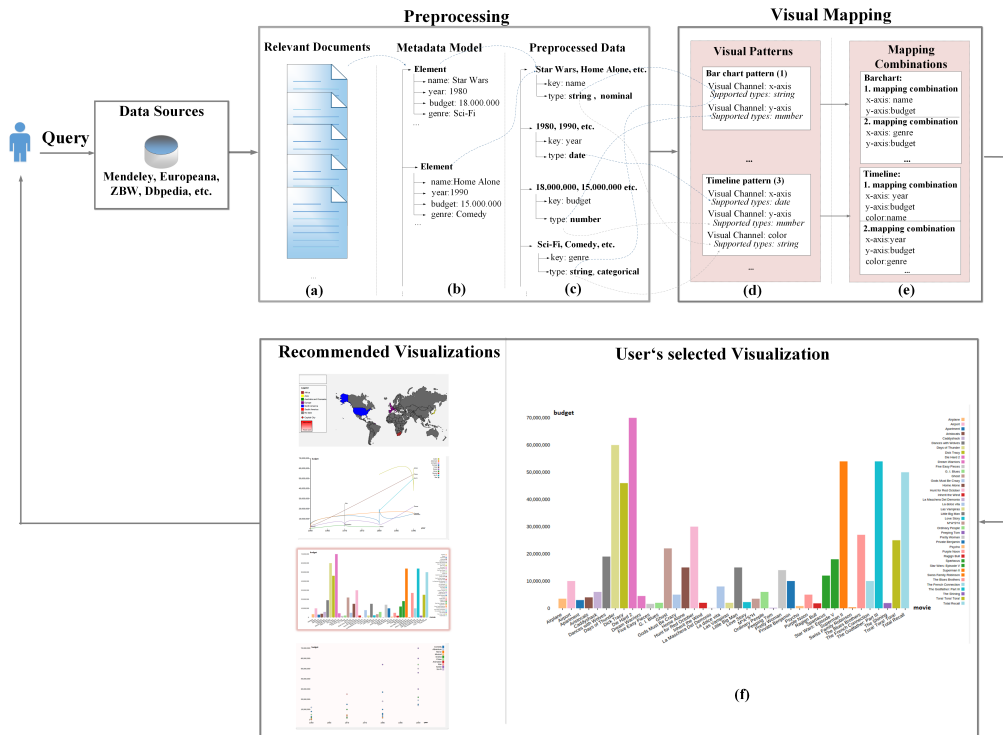
Figure 3.4: Schematic representation of the rule-based recommender: The stages (a), (b) and (c) illustrate the preprocessing unit. The stage (d) illustrates the visual mapping process between the elements and the visual patterns, whereby the defined mapping combinations are shown in stage (e). Finally, the recommendations will be presented to the user in a random order (f).
