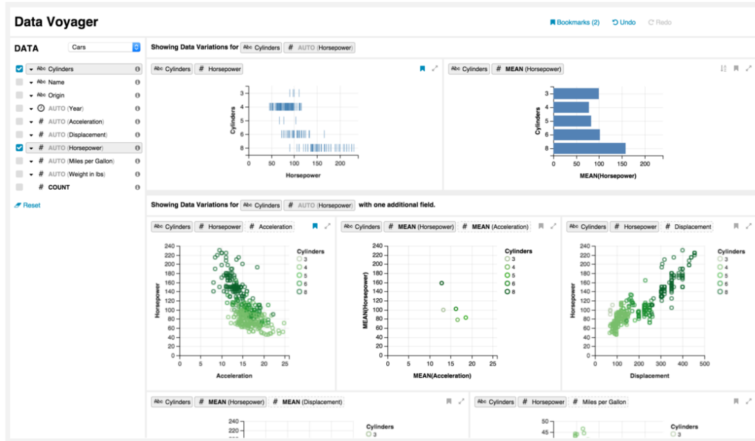
Figure 2.19: The Voyager user interface: The schema panel (left) lists the user-selected attributes. The main gallery (right) presents recommended visualizations of different attribute subsets and transformations. From [WMA + 16], Figure 1.
