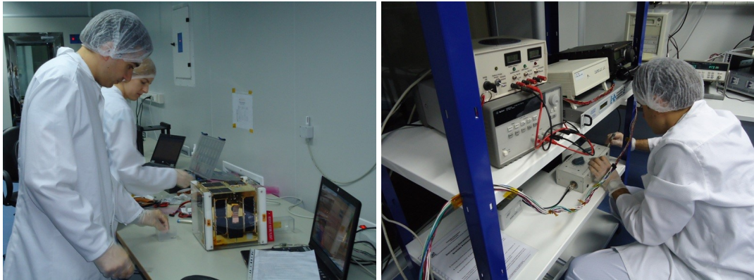
Figure 3.37: Pre-TVAC testing: Before starting with the TVAC testing, the spacecraft had to be functionally tested and the ground support equipment set up and configured.
