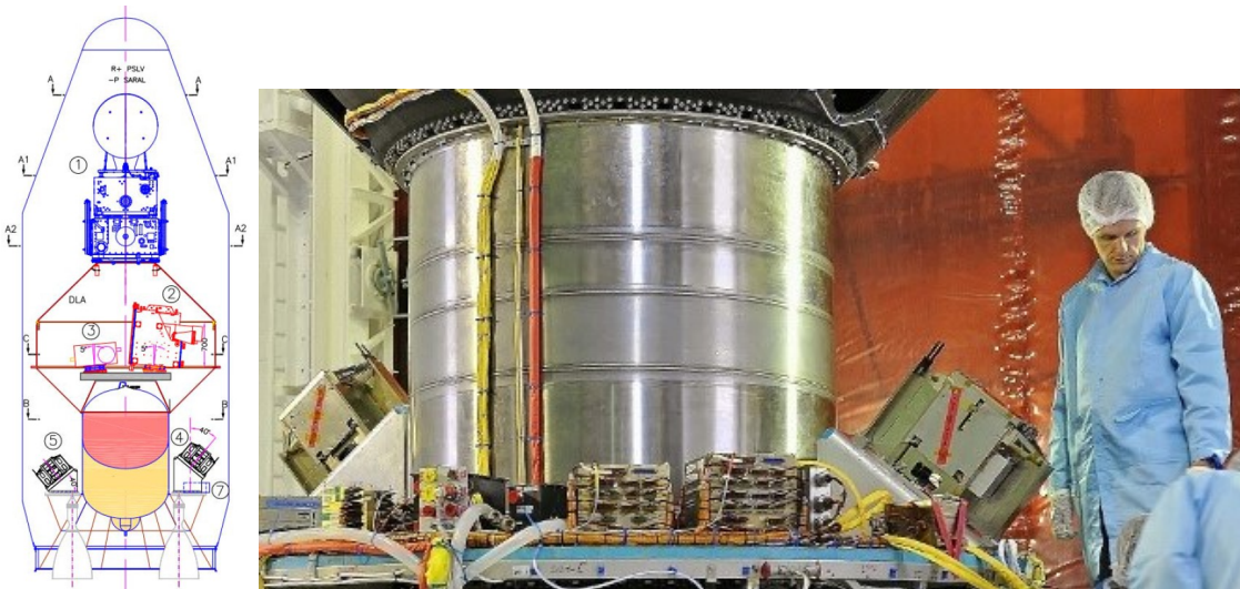
Figure 4.13: Final integration on PSLV: The location of all satellites on the upper stage is depicted (left); An impression of BRITE-Austria (next to C. Grant) shortly before launch is shown (right). (Image courtesy: ISRO)
