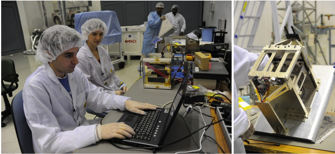
Figure 4.7: Last functional tests and fit check: Before the flight integration of the satellite into its deployer could occur, a final functional check was conducted including software loading. Besides, a fit check of the deployment system on its adapter plate of the payload fairing was performed.
