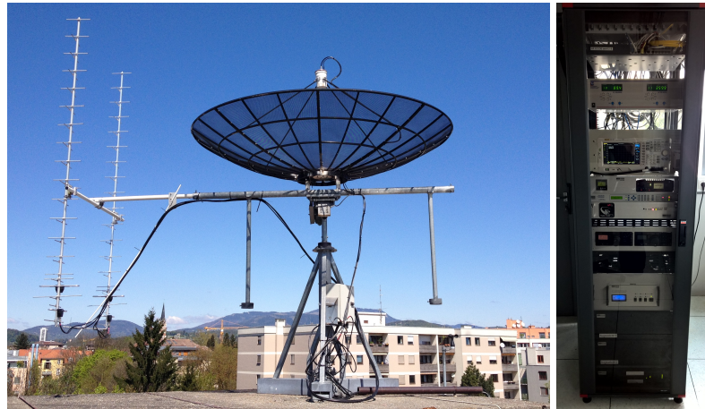
Figure 2.18: Ground station in Graz: Antenna tower and indoor RF equipment used for operations of BRITE-Austria/TUGSAT-1, located at the IKS/TUGraz.
