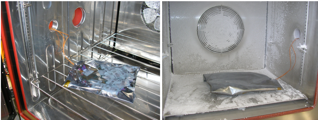
Figure 3.5: Thermal shock testing: Thermal shock testing was performed during the unit-level test campaign on several components (power board is shown).
