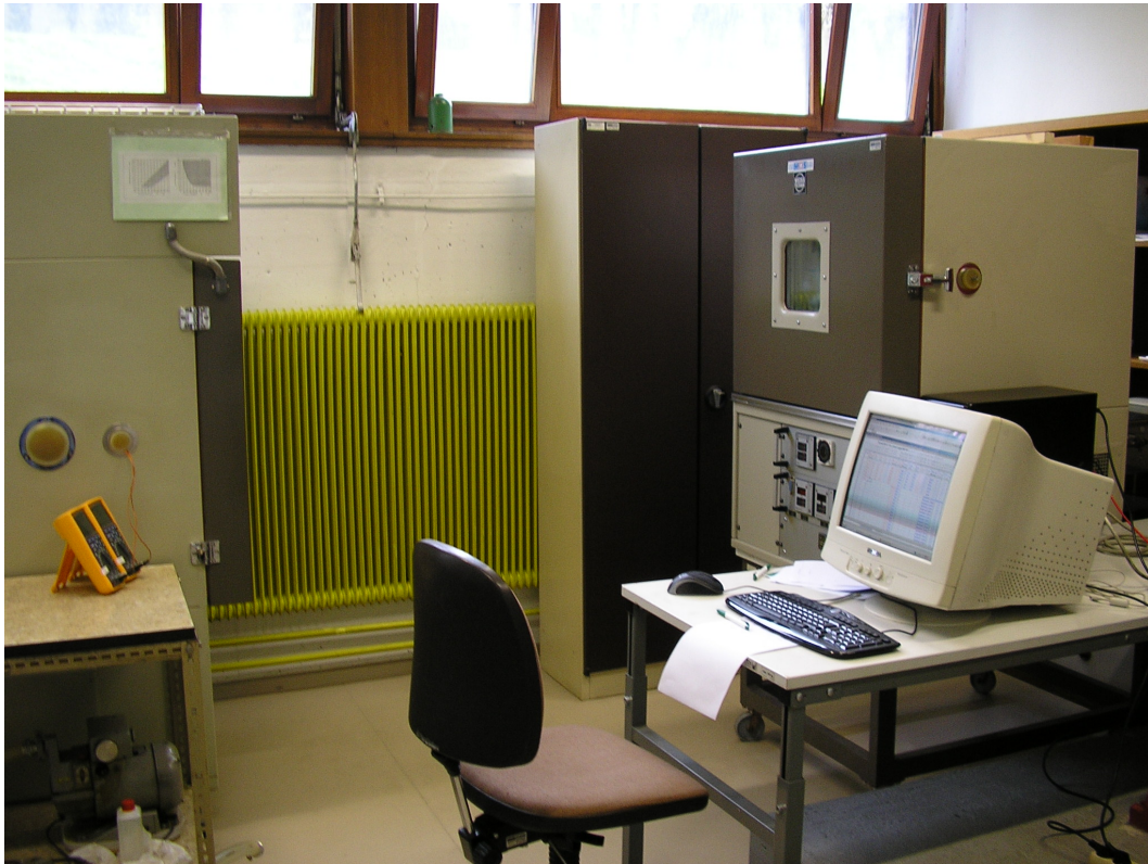
Figure 3.6: Test setup with two chambers for thermal shock testing: Two chambers were used to represent the hot- and cold-case, to ensure the temperature transition of at least 25° C per minute.
