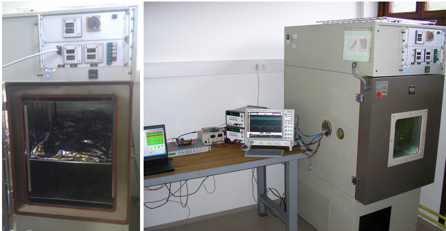
Figure 3.9: Flatsat thermal testing: The functionality of the flatsat was tested at extreme operational temperatures in the thermal chamber.
