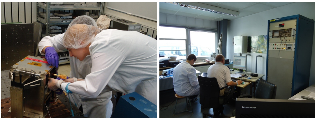
Figure 3.31: Vibration testing: To test a representative flight configuration, the UHF antennas were attached and the test port cover installed (left). In the meantime, the test profile was prepared in the room nearby (right).
