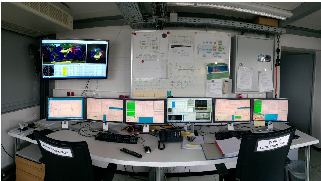
Figure 2.19: Mission control centre in Graz: Several workstations are used for operations of the BRITE-Austria satellite. Starting from the left side, the first three screens are used for operating BRITE-Austria. The fourth monitor shows the ground station interface, while the fifth and sixth screens state the software modules to operate UniBRITE.
