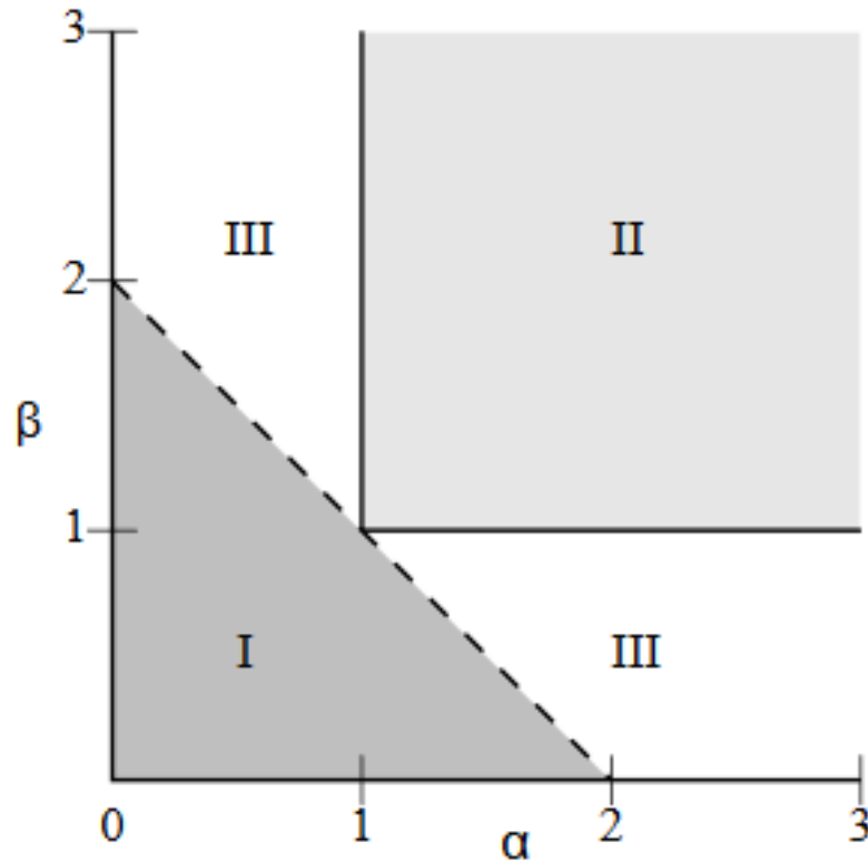
Figure 3.5: Three different system dynamic possibilities (I): \alpha + \beta < 1 three agent coexistence, system is in stable equilibrium (II): \alpha + \beta > 2 and \alpha, \beta \geq 1 , single agent equilibriums are stable; (III): \alpha + \beta \geq 2 , and \alpha or \beta \leq 1 there is no possible stable equilibrium point, only a periodic orbit
