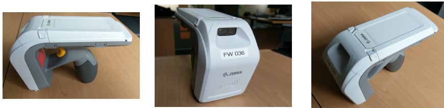
Figure 5.1: The RFID reader I used for my experiments. It is a ZEBRA RFD8500 Handheld with maximum power of 30 dBm, which is equal to 1W. I operate the reader at Session 0 in AB flip mode.
