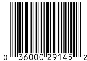
Figure 2.1: Example of a bar code in the form of a universal product code (UPC). The reader needs a direct line of sight to read the code, as it needs to traverse the pattern perpendicular to the bars.
