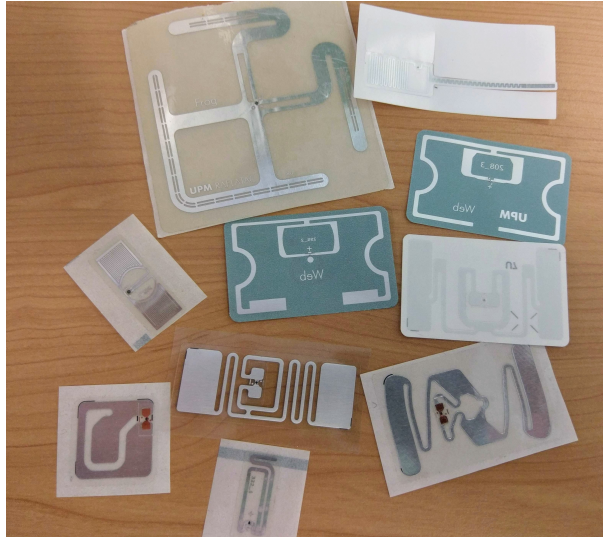
Figure 2.2: Examples of passive RFID tags.
