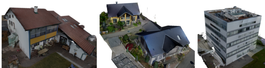
Figure 3.4: Outputs of the reconstruction with plane based regularization. It can be seen that the planar surfaces on the buildings have been densely reconstructed. Figure taken from [25].
